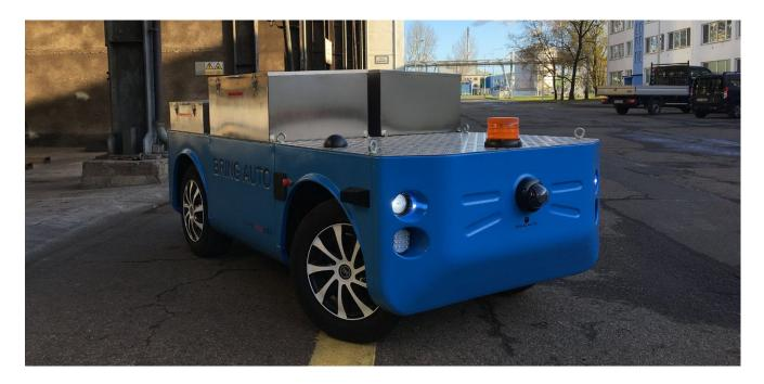
The Delivery Robot has electrically driven rear axle (Benevelli motor), standard option 48V lead battery (330 Ah) provides operation time up to 10 hours for single charge. Onboard 230V charger allows for recharging the battery within 5 hours (10% to 90%). Optional lithium-ion battery pack available.
